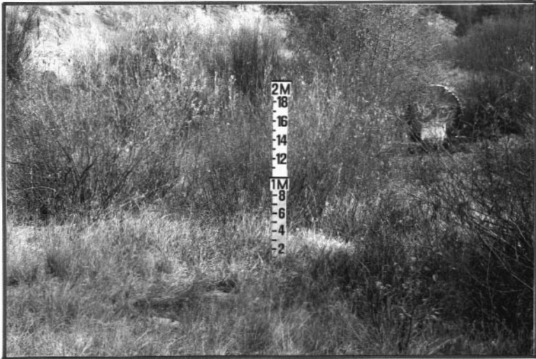
Figure 21—Use of a folding 2-meter board to document height and growth of tall shrubs. This board is hinged in the middle and held upright by a barrel bolt. When folded together (fig. 54, part B), it is a 1-meter board and unfolded it is 2 meters.
