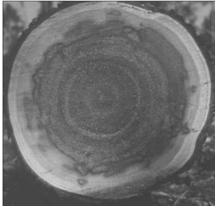
Fig. 10. Advanced red-brown decay in Douglas-fir, with spindle-shaped white pockets, caused by Fomes pini
