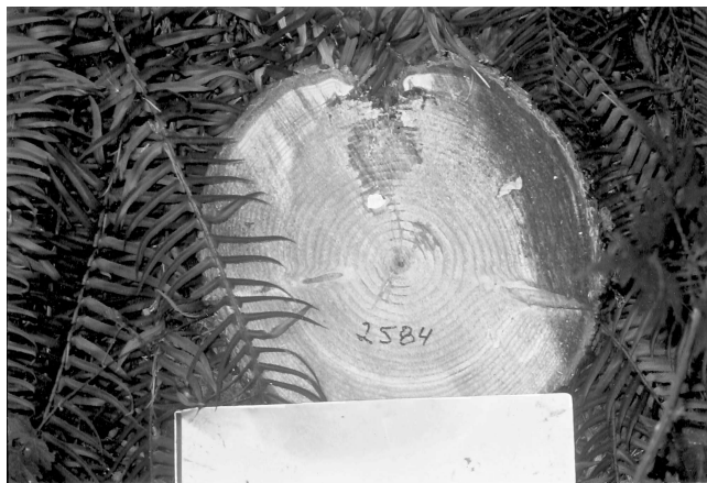
Figure 1. Trunk wound (top of disk) at about 8 m aboveground caused by a fungal-inoculated rifle bullet (white spot below stain) and subsequent wood decay (stain) in a live Douglas-fir inoculated 5 years previously.
