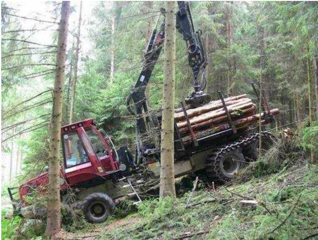
Figure 6: Herzog Forcar FC200 8x8 winch-assisted steep slope forwarder working in southwest Germany.
