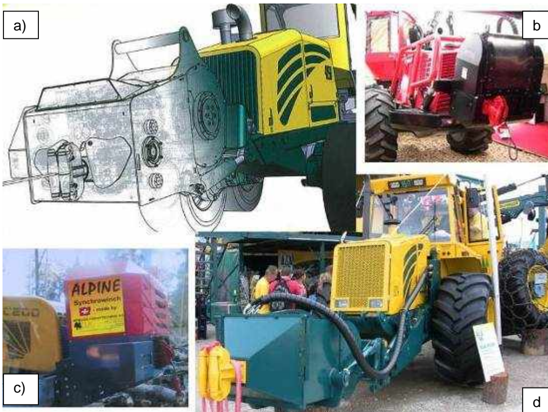
Figure 12: CAD drawing a) and photo d) of the HSM Slope Terrain Winch (HSW-15). Photo b) of traction winch manufactured by Ritter; Photo c) Alpine Synchronwinch manufactured by Herzog Forsttechnik.
