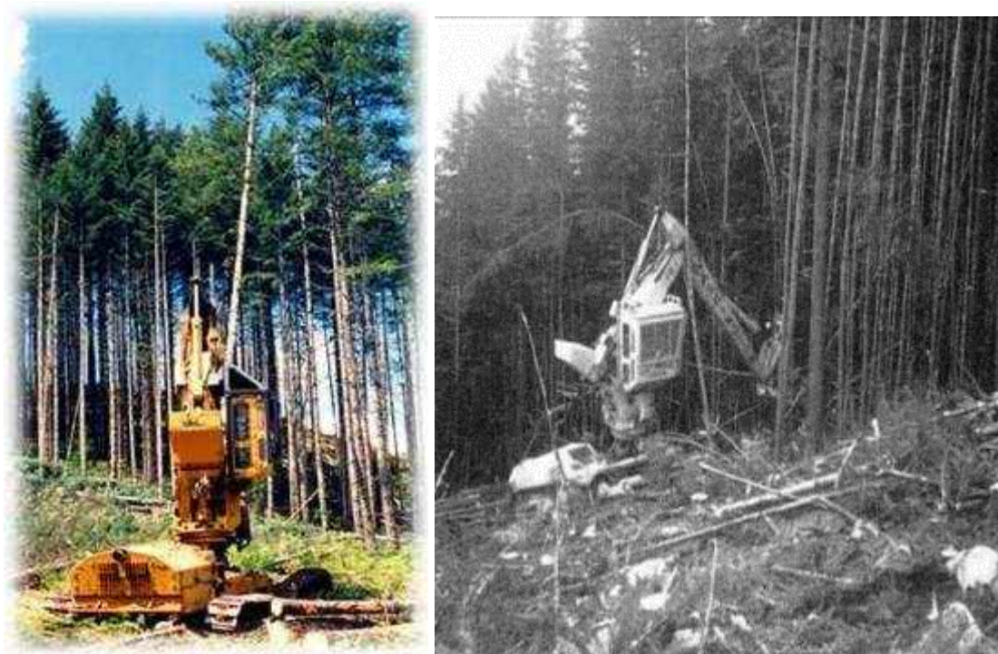
Figure 3: The ATH28 Allied Tree Harvester reportedly worked comfortably on relatively steep slopes
