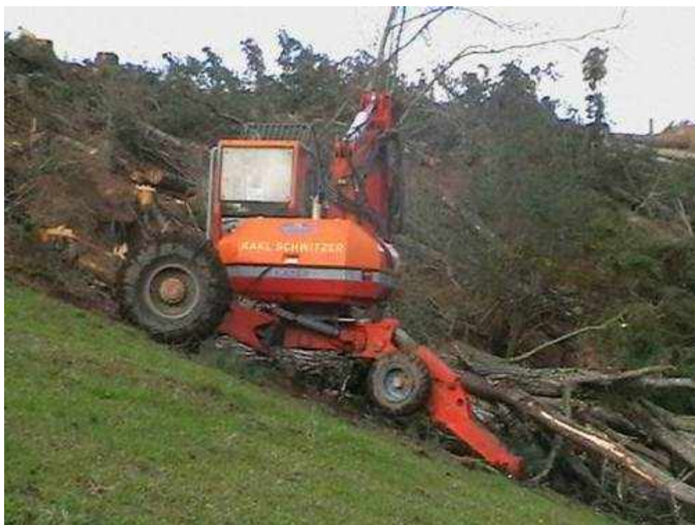
Figure 4: Side view of Kaiser Spyder showing degree of cab levelling possible. Note stabiliser angle which illustrates the reliance on the stabiliser penetration for stability.
