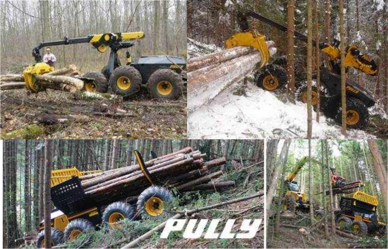
Figure 9: Operation of the Konrad Pully.
