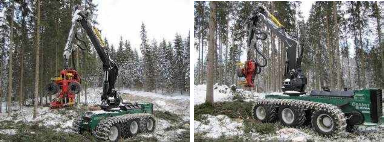
Figure 7: Teleoperated harvester Greemo Besten 106 RH
