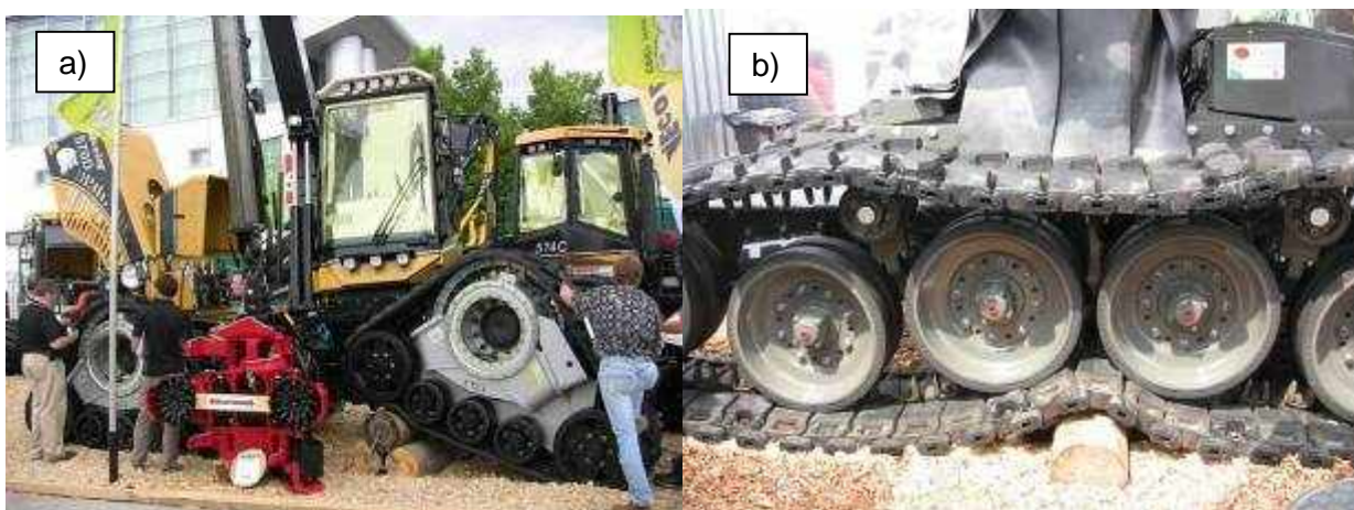
Figure 13: Available options for improved track performance: a) the WFW's SoftTrack drive and b) flexible track concept (Street Rubbers) by Impex Königstiger.
