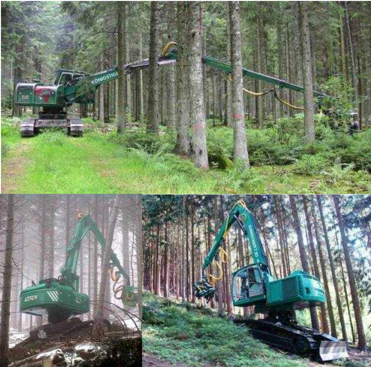
Figure 5: Excavator-based Impex Königstiger Harvester working in a selection cutting in Southwest Germany.
