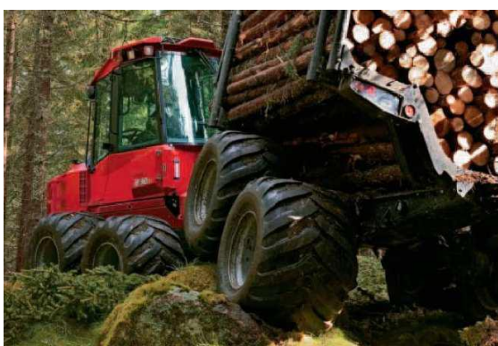
Figure 50: Showing the advantage of a passive bogie wheel as the vehicle negotiates over a boulder. (Hellström et al., 2008)
