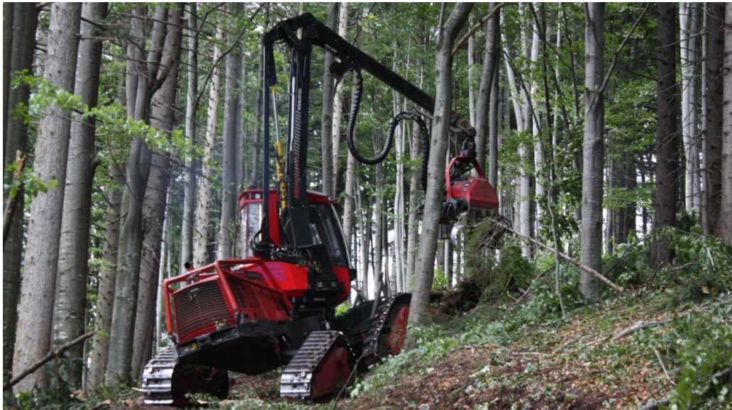
Figure 49: Komatsu 911 Snake harvester showing the advantage of passive bogie quad tracks. Note how the front visible track is on a different plane to the two rear tracks however all tracks are in full contact with the ground.
