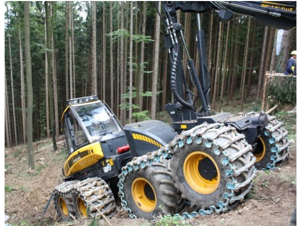
Figure 8: Ponsse Ergo 8 with bogie tracks over all 4 pairs of bogies
