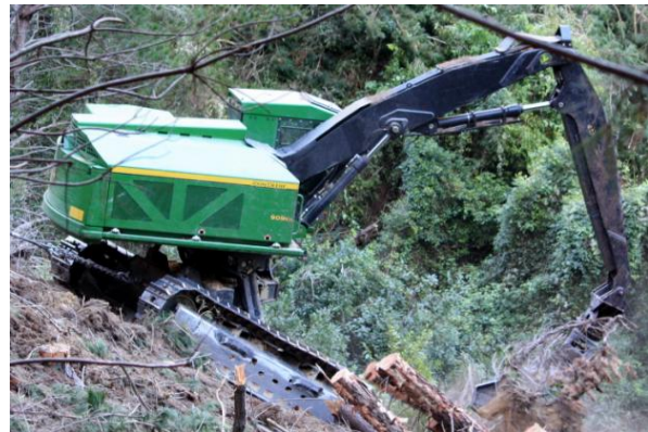
Figure 10: John Deere 909KH self levelling harvester working tethered using a wire rope.
