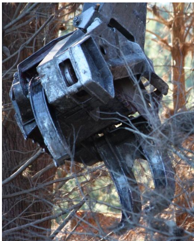
Figure 3: Felling head considerably lighter than the alternative processing head consisting of a grapple and a bar saw.
