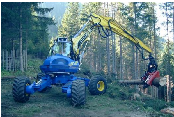
Figure 6: Kaiser S2 4x4 Cross walking excavator with each wheel able to raise or lower individually 2
