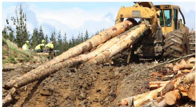
Figure 15: Soil damage from skidder wheels and skidded logs
