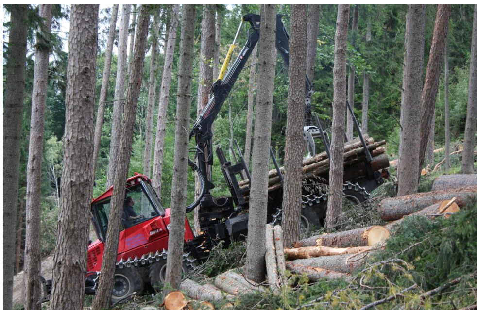
Figure 11: Forwarder operating on moderate slopes in Austria, note the log piles of equal length logs in this cut to length system. This machine was following through a stand that had been felled with a harvester and subsequently is driving on slash rather than the topsoil.
