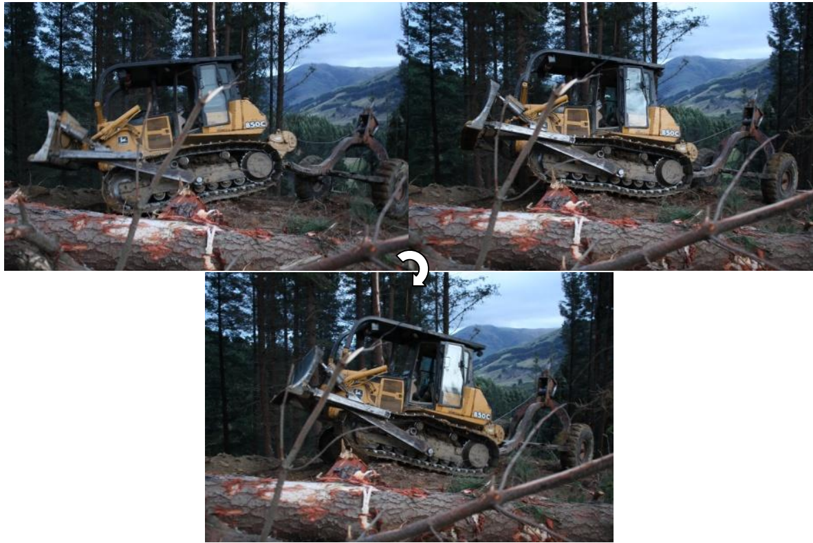
Figure 52: Photo series of a rigid track bulldozer reversing over a stump, note the rapid change in the machine slope over a relatively short distance.
