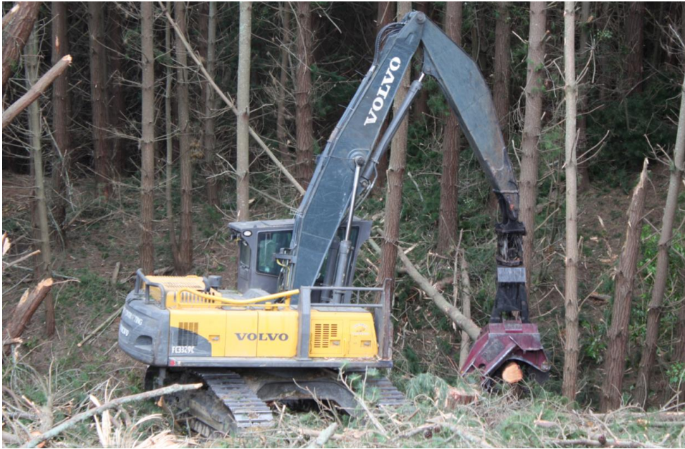
Figure 1: Volvo excavator felling in small piece size pine plantation. Note the rigid track based undercarriage and the housing that can rotate on top of the undercarriage.
