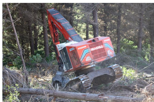
Figure 51: Showing a rigid track machine experiencing excessive slope due to an obstacle.
