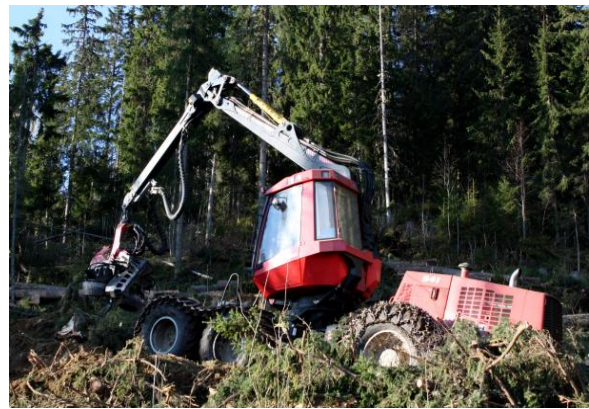
Figure 9: Komatsu 941 harvest equipped with front bogie tracks and chains on the rear wheels
