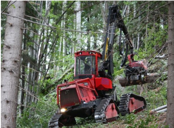
Figure 5: Komatsu 911 Snake harvester operating in a mixed forest in Central Austria
