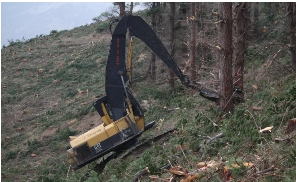
Figure 2: A typical New Zealand felling machine. These machines have a reinforced cab to meet forestry equipment regulations and often have a widened and lifted track base to increase clearance.
