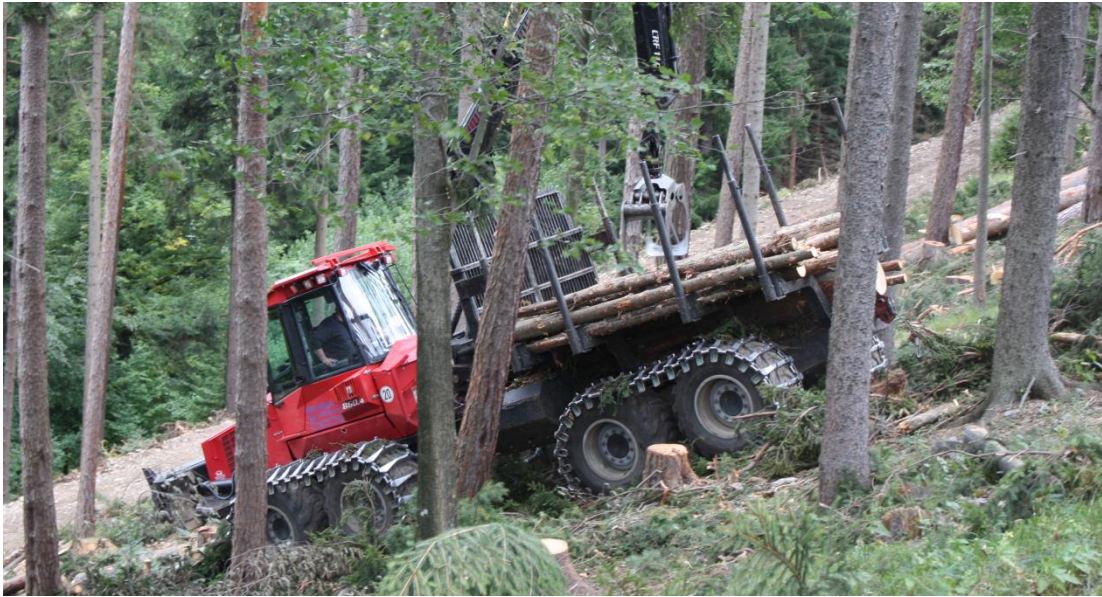
Figure 53: An eight wheeled forwarder in Austria working on steep terrain operating down slope as it loads its bunk and then reversing back uphill when empty.
