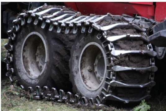
Figure 14: Steep terrain bogie tracks
