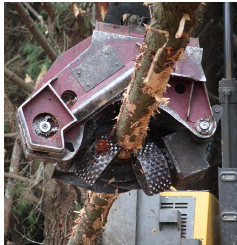
Figure 4: Processing head, note the large rollers that are absent on the felling head. The head is also fitted with knives (behind the rollers) for removing limbs and bark.
