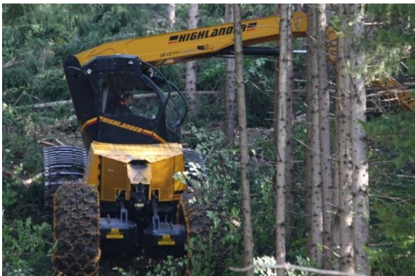
Figure 7: Konrad Highlander 6w - A purpose built steep terrain European harvester
