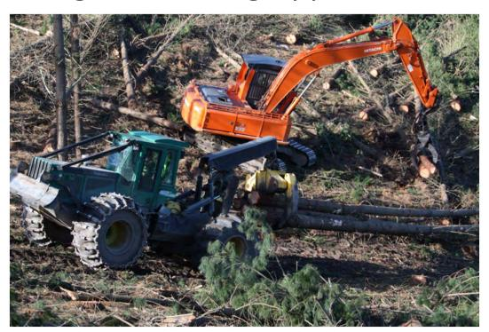
lifted and widened track base and modified cab for better vision and improved protection.
