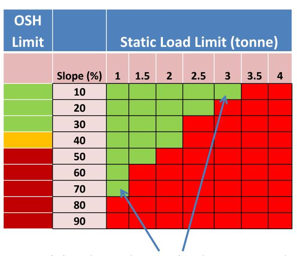
Static stability dependant on load position and machine type (MacLean & Visser 2011)
