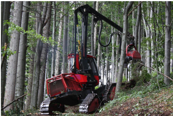
Figure 5: Komatsu 911 Snake harvester showing the advantage of passive bogie quad tracks.
