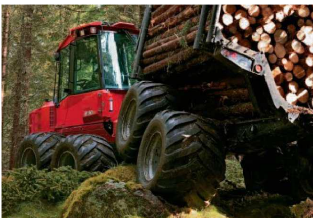
Figure 6: Showing the advantage of a passive bogie wheel as the vehicle negotiates over a boulder.
