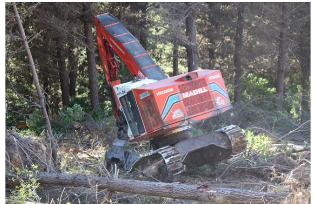
Figure 7: Showing a rigid track machine experiencing excessive slope due to an obstacle.
