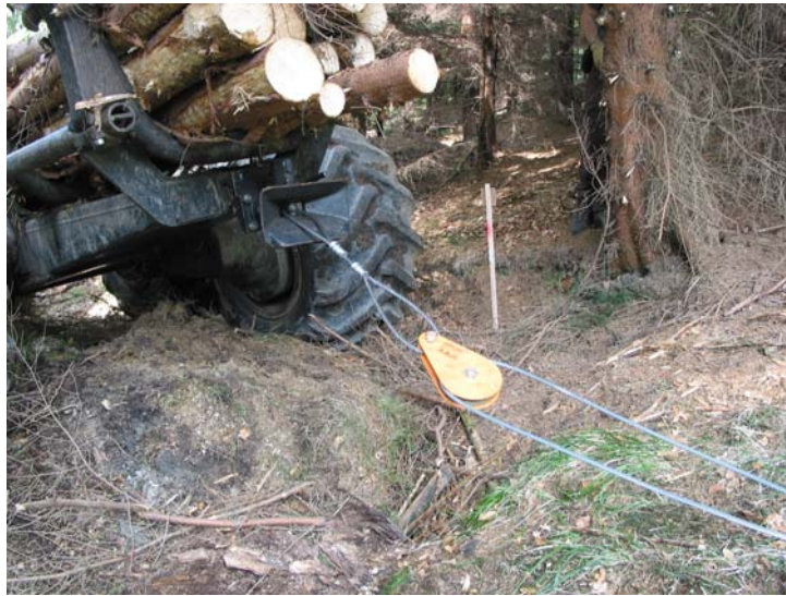
Figure 2: Rear tow – bar of the forwarder and traction rope
