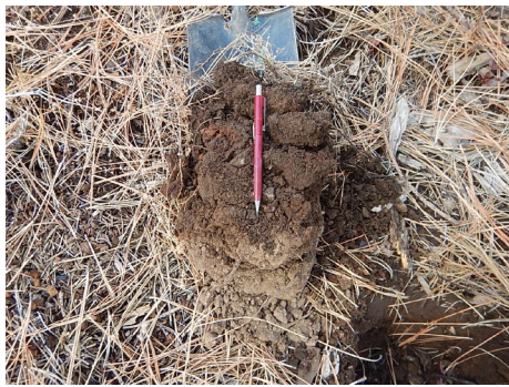
Fig. 11: Platy compacted soils.
