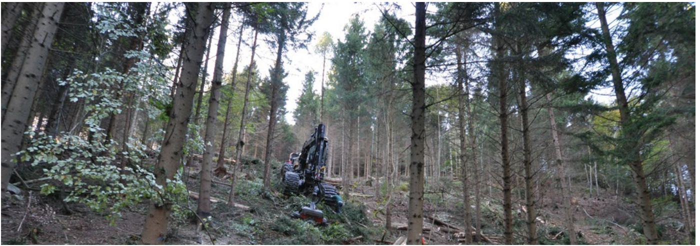
This harvester is a wheeled winch assist machine working on a 75 per cent slope in the Swiss Alps in a cut-to-length thinning operation.
