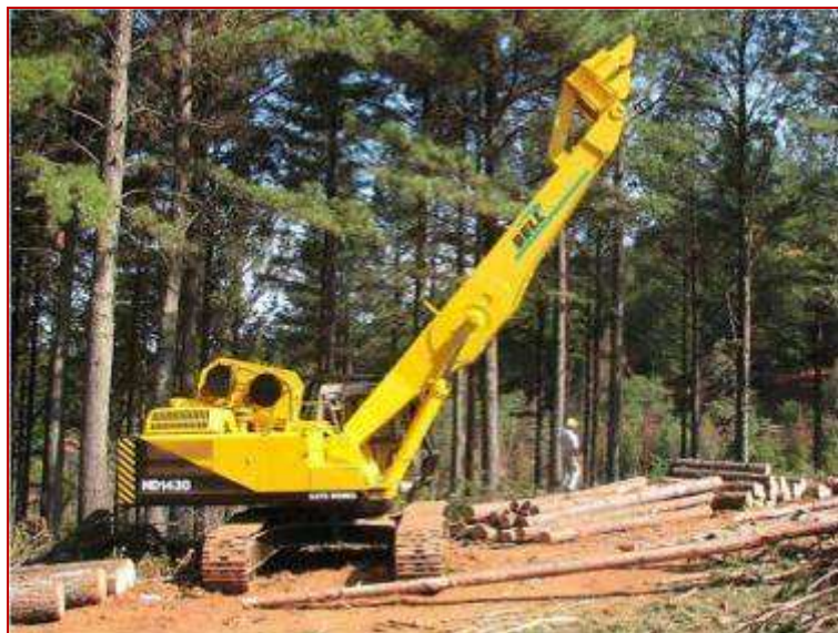
Figure 16. Excavator based cable yarder ( www.loggingon.net )
