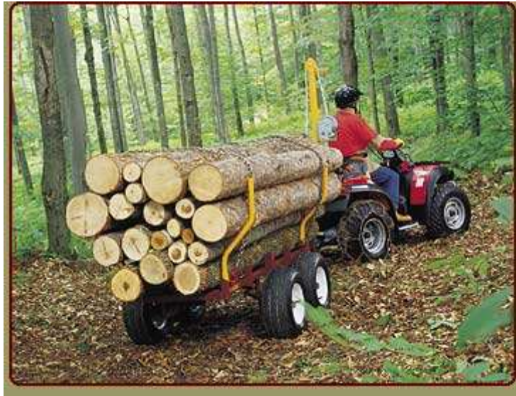
Figure 47. ATV with log trailer with a bogie axle ( www.novajack.com )
