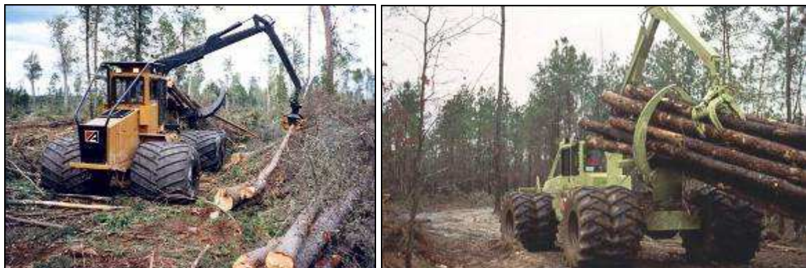
Figure 21. High flotation and dual tyres on clambunk skidders ( http://nrs.fs.fed.us/ )
