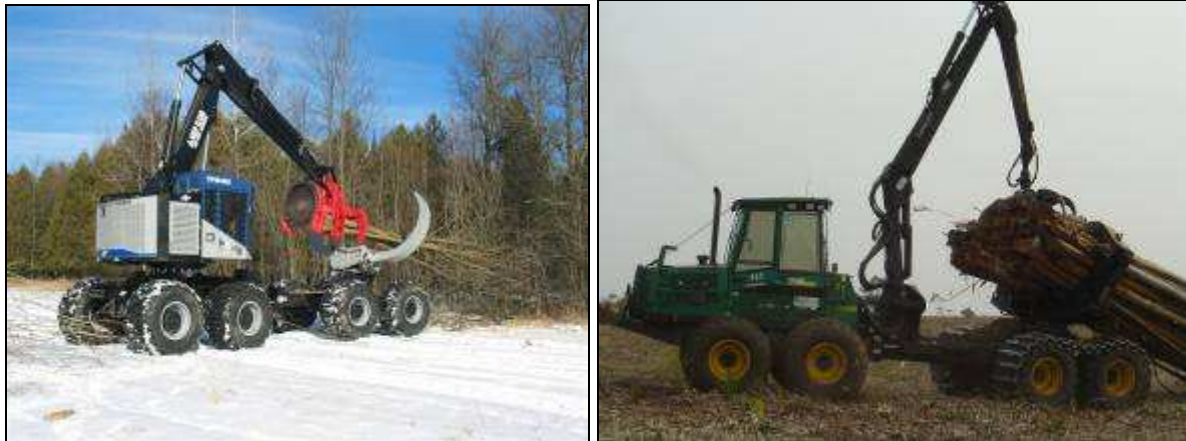
Figure 13. Timberpro 840 Feller buncher clambunk skidder combo ( www.timberpro.com ) and John Deere 1710D clambunk skidder
