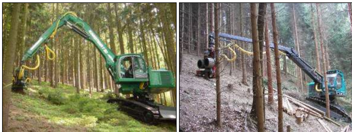
Figure 26. Harvesters with a levelling upper structure ( www.impex-forstmaschinen.de and www.neuson-ecotec.com )
