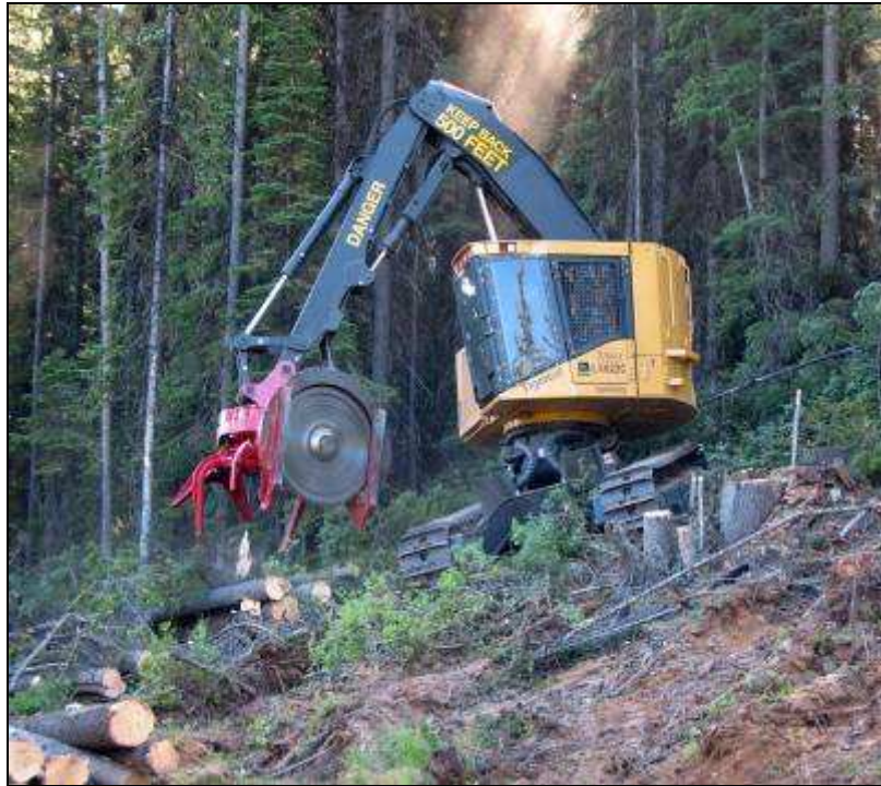
Figure 34. Feller buncher with high rotation head ( www.tigercat.com )
