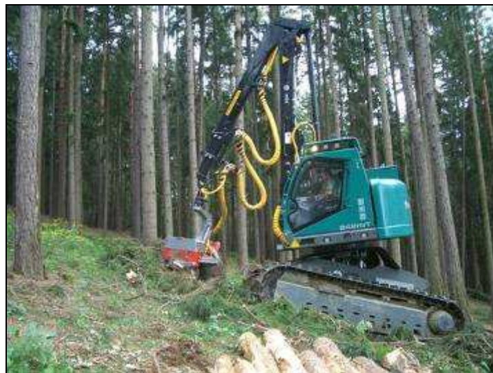
Figure 4. 242HVT tracked harvester ( neuson-ecotec.com )
