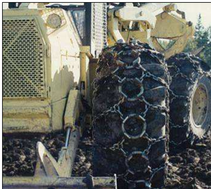
Figure 23. Tyre chains with rings ( www.babactirechains.com )
