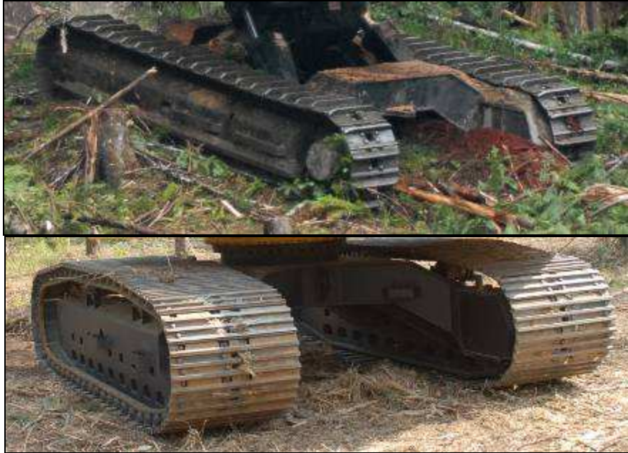
Figure 24. Single and triple grousers, and traction and flotation tracks ( www.tigercat.com )
