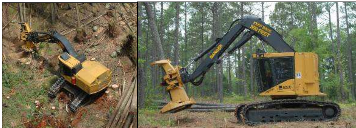
Figure 28. Tail swing vs. zero tail swing ( www.tigercat.com )
