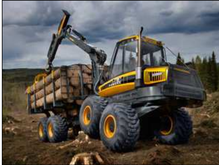
Figure 20. Bogie axle driving over stump ( www.ponsse.com )
