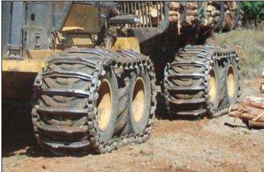
Figure 22. Traction band tracks fitted to a forwarder
