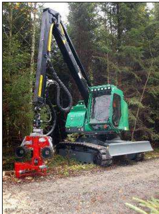
Figure 30. Skidding blade fitted to a tracked harvester ( www.neuson-ecotec.com )
