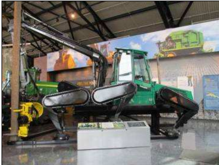
Figure 43. John Deere walking harvester ( www.JohnDeere.com )
