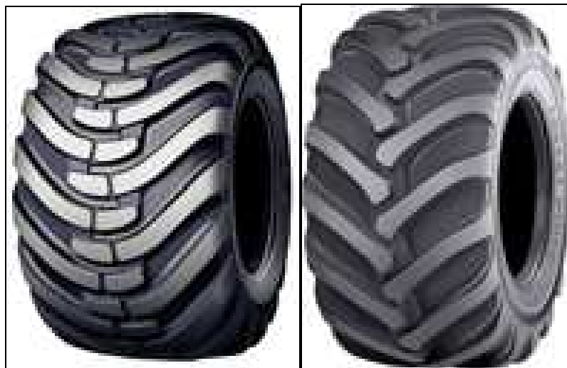
Figure 18. Flotation vs. traction tyres ( www.nokianheavytyres.com )
