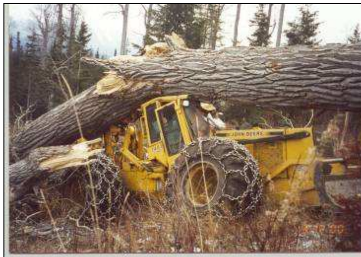
Figure 1. Effectiveness of FOPS and ROPS structures ( http://customproductsinc.files.wordpress.com/2011/10/skidder-versus-tree.jpg )
