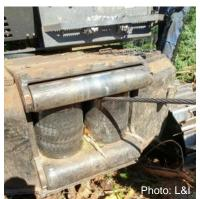
The ClimbMAX system has a single wire rope with an internal drum. The wire rope is anchored directly to a tree, stump, or another fixed structure.
