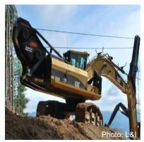
Tractionline is a dual wire rope auto-tension system. The two drums are mounted on a base machine that is positioned uphill and communicates with the tether machine via radio signal.
