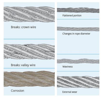
Examples of common wear and defects in wire rope
