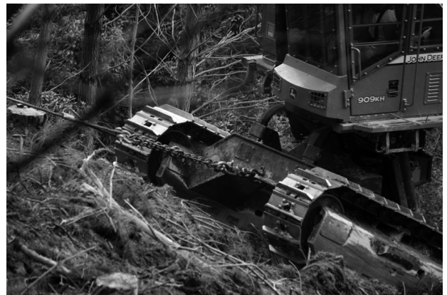
Fig. 12 Chain used for last section to prevent wear and tear on cable (photo from Hamish Berkett)
