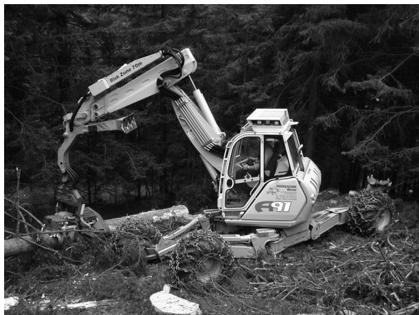
Fig. 4 Menzi Muck A91 as an example of a harvester with wheels on hydraulically actuated »arms« that can lower its centre of gravity to improve stability (photo from Raffaele Cavalli)
