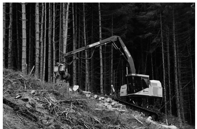
Fig. 2 Tigercat steep terrain feller-buncher shows that self-levelling cab feature is also used to redistribute the weight uphill for increased stability
