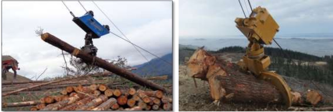
Figure 5: 'Motorised' grapple carriages; Falcon Forestry Claw with internal motor (left), and hydraulically powered Alpine (right).
