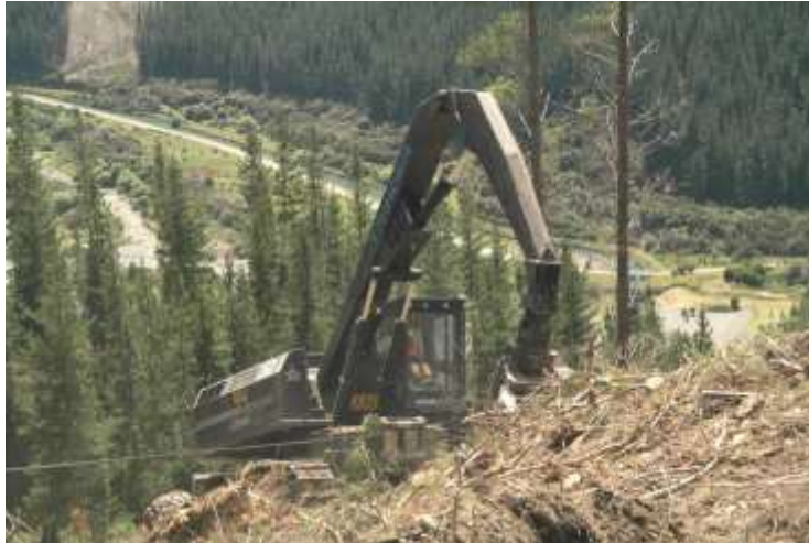
Figure 2: ClimbMAX felling machine with integrated winch mounted on chassis
