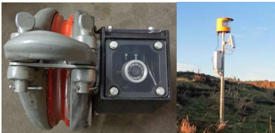
Figure 6: Left, camera mounted on a block that is towed by a carriage or rider block along the skyline. Right, camera mounted in the cutover. Both cameras transmit a video signal back to the yarder cab to assist the operator with the grapping task.
