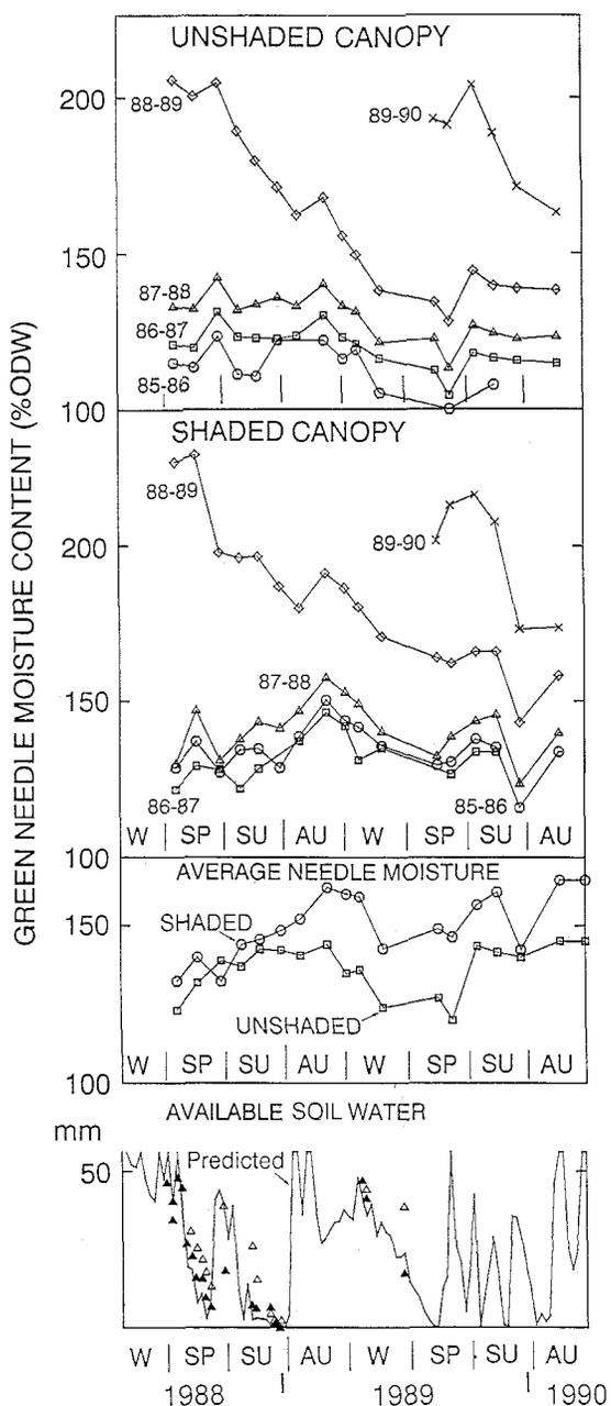
**Figure 7.** Seasonal changes in the moisture content (LFMC) of different aged cohorts and the average moisture content of green needles from shaded and unshaded locations in *P. radiata* canopies shown in relation to the water balance of topsoils. Needle cohorts and their ages are identified by the growth season of their production e.g. '88-'89.
